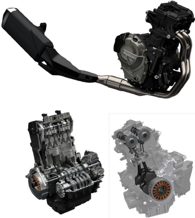
776cc, four-stroke, liquid-cooled, DOHC, parallel twin engine
