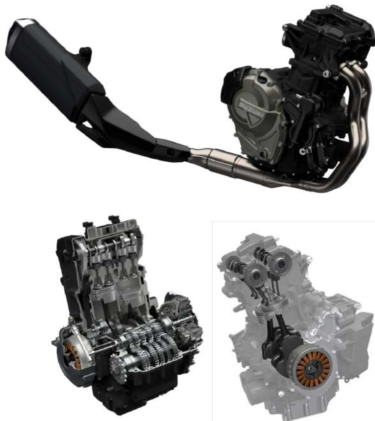
776cc, four-stroke, liquid-cooled, DOHC, parallel twin engine
