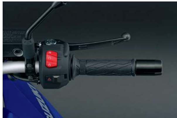
Right handlebar switch
