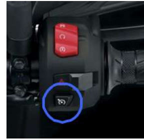
Right handlebar switch
