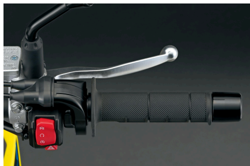
Right handlebar switch
