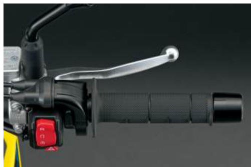
Right handlebar switch
